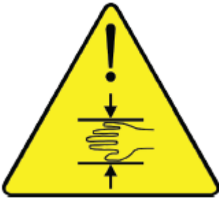
2. Warning decal, risk of crushing
