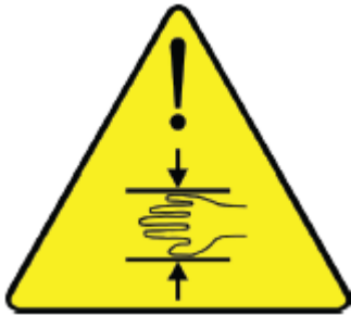
2. Warning decal, risk of crushing
